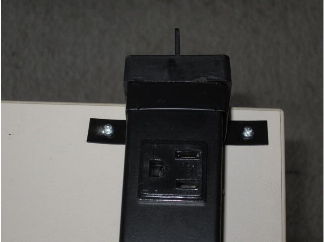
Figure 5-6. The power strip is fastened securely to the table using the provided hardware. You do not want your power strip wiggling around, or worse yet, falling off the table, dragging all of your power tools with it!
