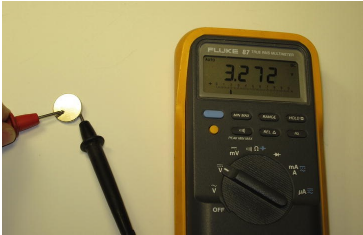
Figure 4-5. Measuring a coin cell’s electrical goodness using a digital multimeter. This one is chock-full of goodness!
