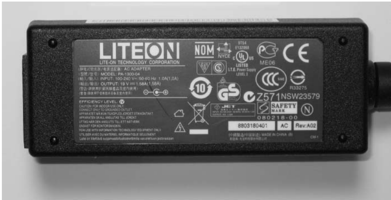
Figure A-4. A name-brand laptop charger with several international safety certifications. Every one of these certifications costs money to obtain, and shows that the device was demonstrated to be safe for use in a typical home or business application.
