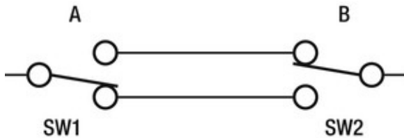
Figure 5-19. A three-way switch circuit built using two SPDT switches. Power is either carried by the upper wire or the lower wire, as long as both switches are in the same position. If not, then no power flows across this part of the circuit. As shown, the three-way switch is effectively off. Flip either switch to turn it on.
