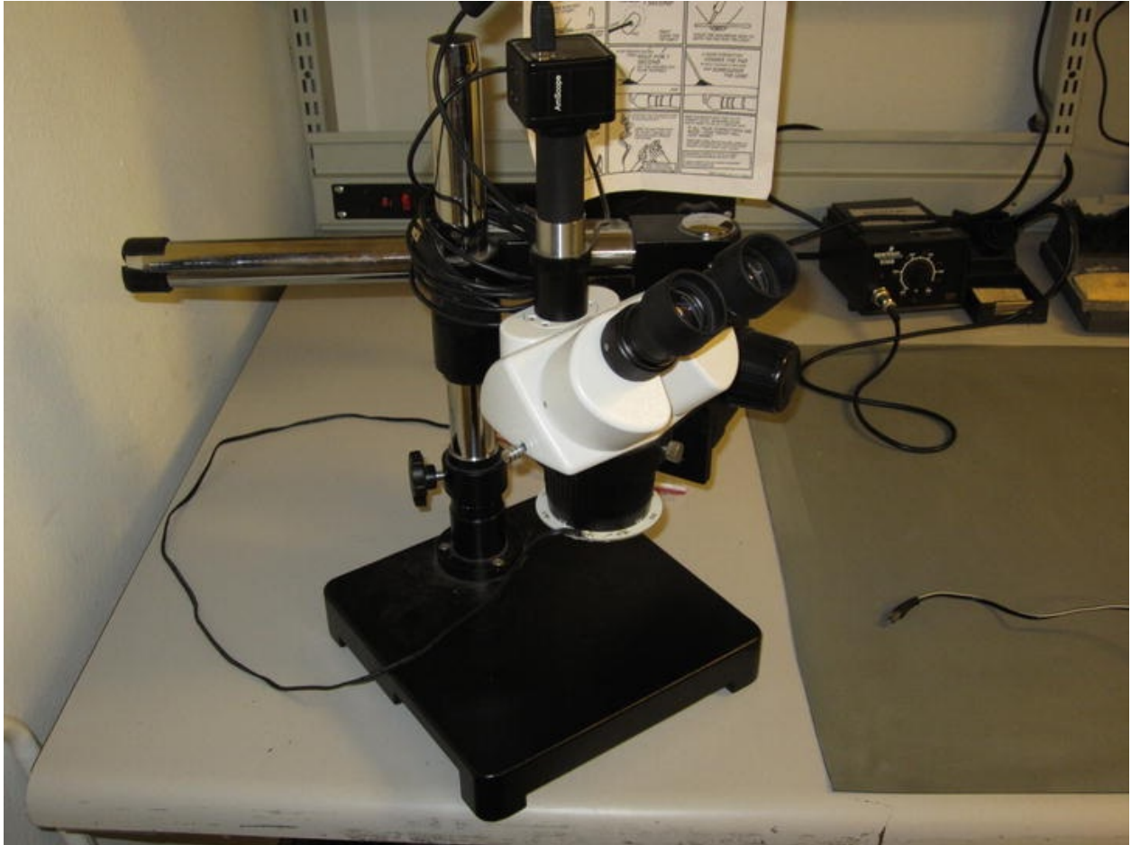
Figure 2-17. A very nice stereo microscope. The power cord running to the white ring (partially hidden) supplies power to a ring of white LEDs that help illuminate the field of view. The base is very heavy to help stabilize the microscope.
