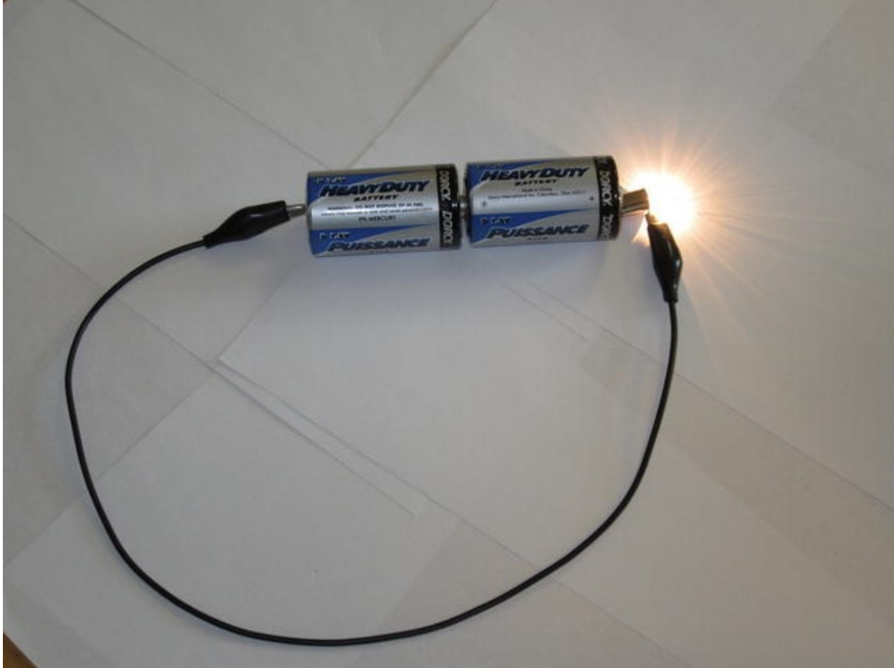
Figure 1-4. The completed circuit, showing the glowing bulb. Electricity is flowing!
