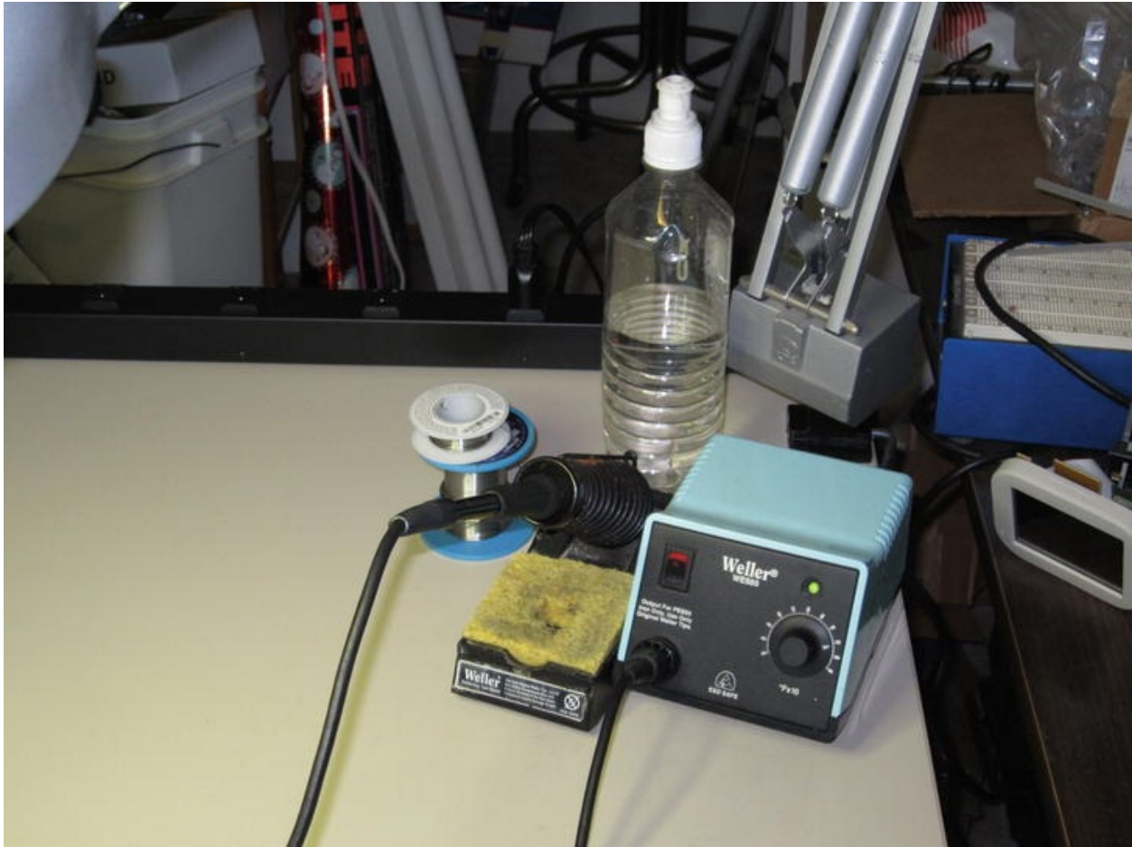
Figure 5-8. A temperature-controlled soldering station with a stand for the soldering iron, a water bottle to wet the tip-wiping sponge, and some different kinds of solder. Some people prefer to have the soldering station nearer to the front edge of the table. Use whatever configuration makes the most sense in your lab.
