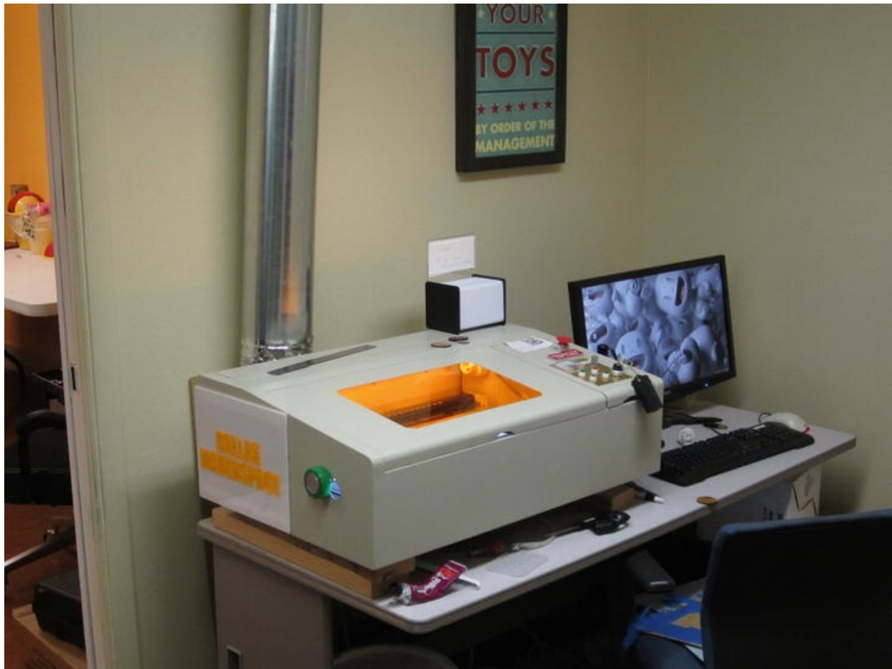
Figure 2-15. A laser cutter. A powerful 40W carbon-dioxide laser is used to cut through wood and non-chlorine-based plastic, all under computer control. It can also be used as an engraver. This model is manufactured by Full Spectrum Engineering.
