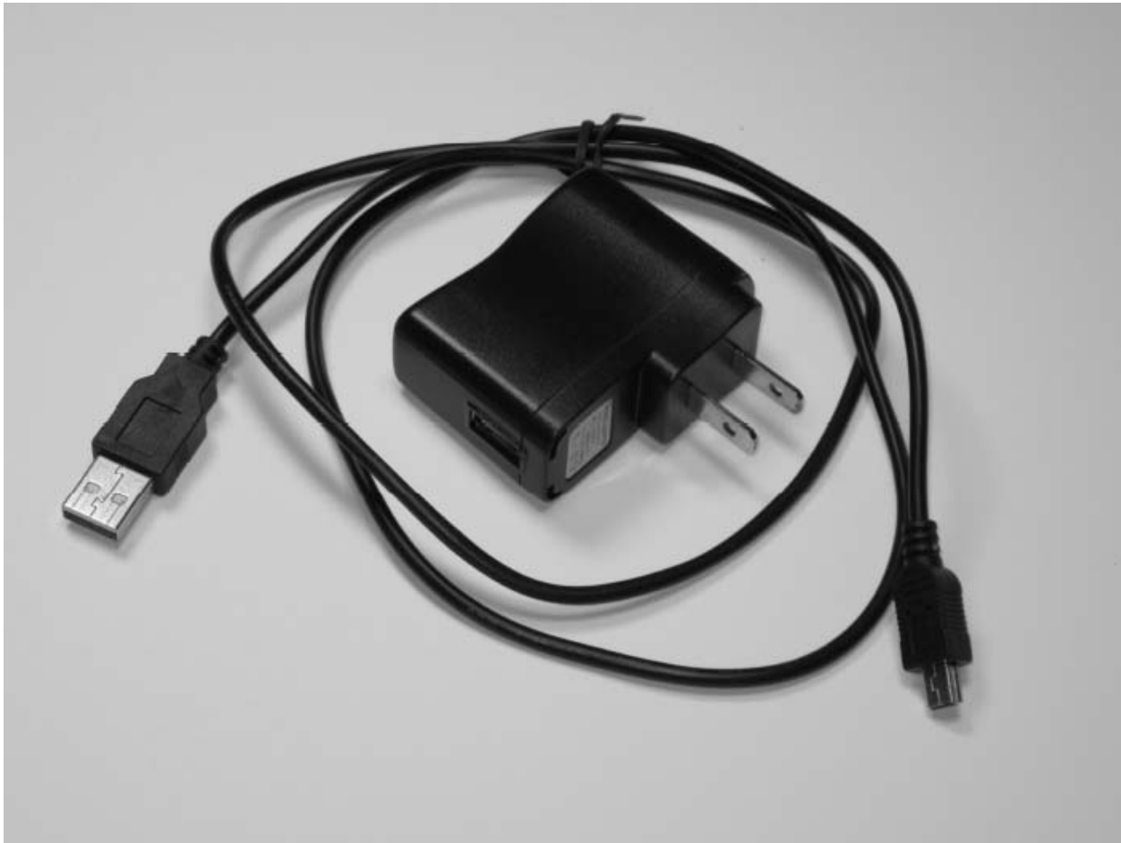
Figure A-2. A USB charger that plugs into the wall and provides a regulated +5V supply. This plug is intended for US wiring, but will operate from 110VAC to 240VAC at 50 or 60Hz, which pretty much covers the whole world, if you have the right adapter plug.
