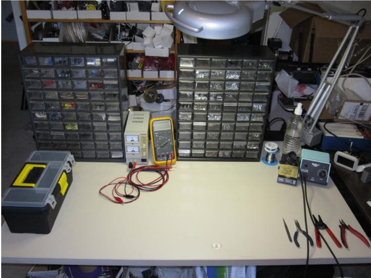
Figure 5-10. Parts bins are used to organize components. This style of container is available in many sizes with different numbers and sizes of drawers. Even more parts are stored on a shelf behind the work area. The most commonly used hand tools are laid out on the right. The other hand tools are collected in a small toolbox on the left.
