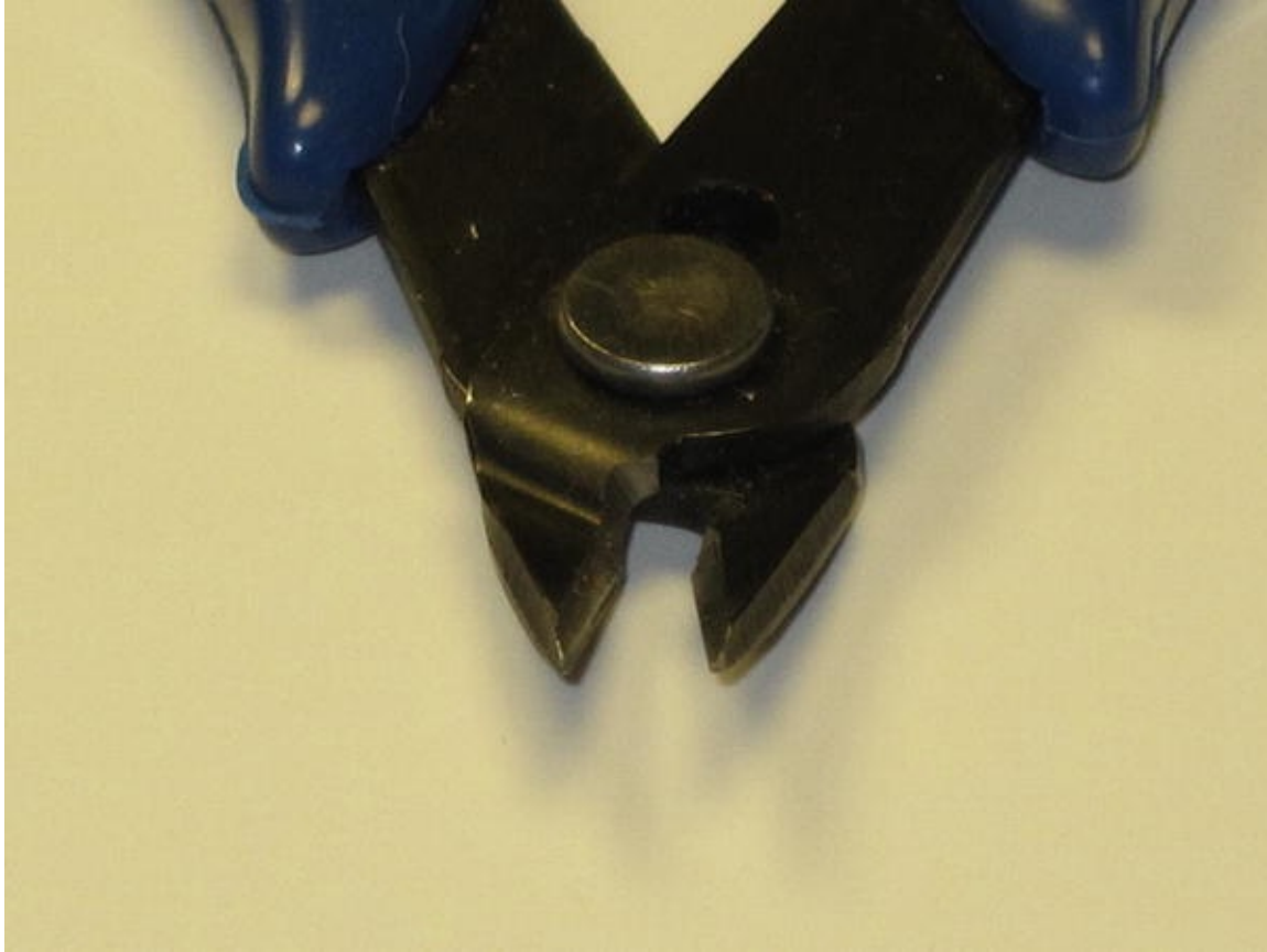
Figure 2-2. A close-up look at the business end of a pair of side cutters. When the two cutting edges meet in the middle, the bottom side is flat, or flush, allowing the user to get quite close to where a wire or component lead emerges from a solder joint.
