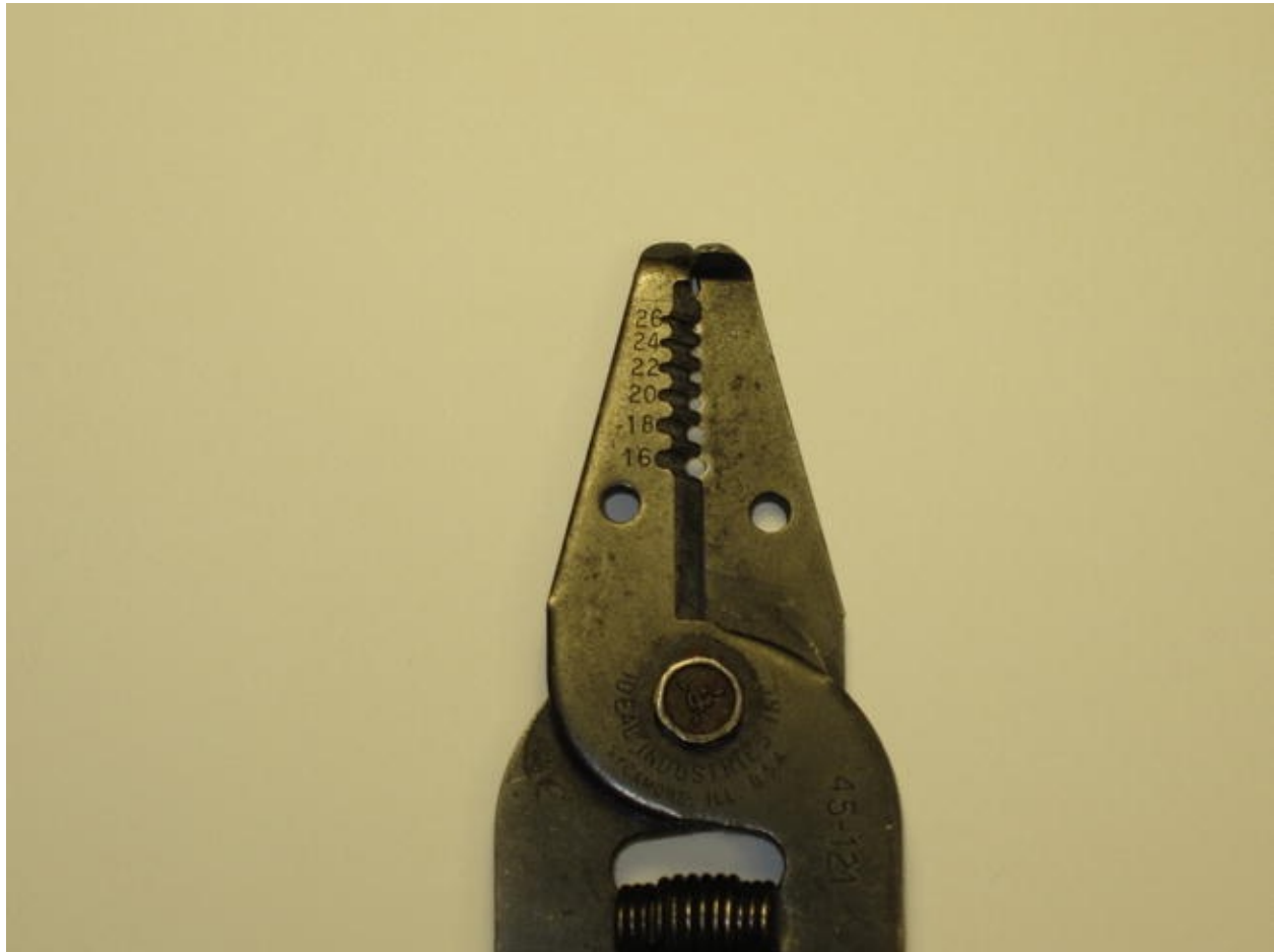
Figure 2-3. The popular T-Stripper combination wire cutter and stripper tool from Ideal Industries has been around for over half a century. Note the wire gauge sizes stamped into the face of the cutter blade. New models feature laser-engraved text.
