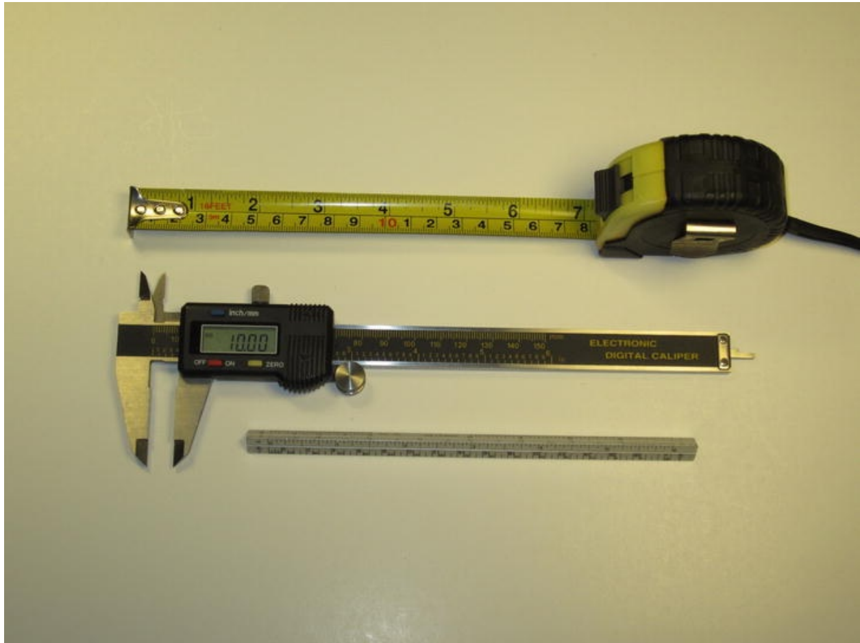
Figure 2-19. From top to bottom, a tape measure, a set of digital calipers, and an architect's scale.
