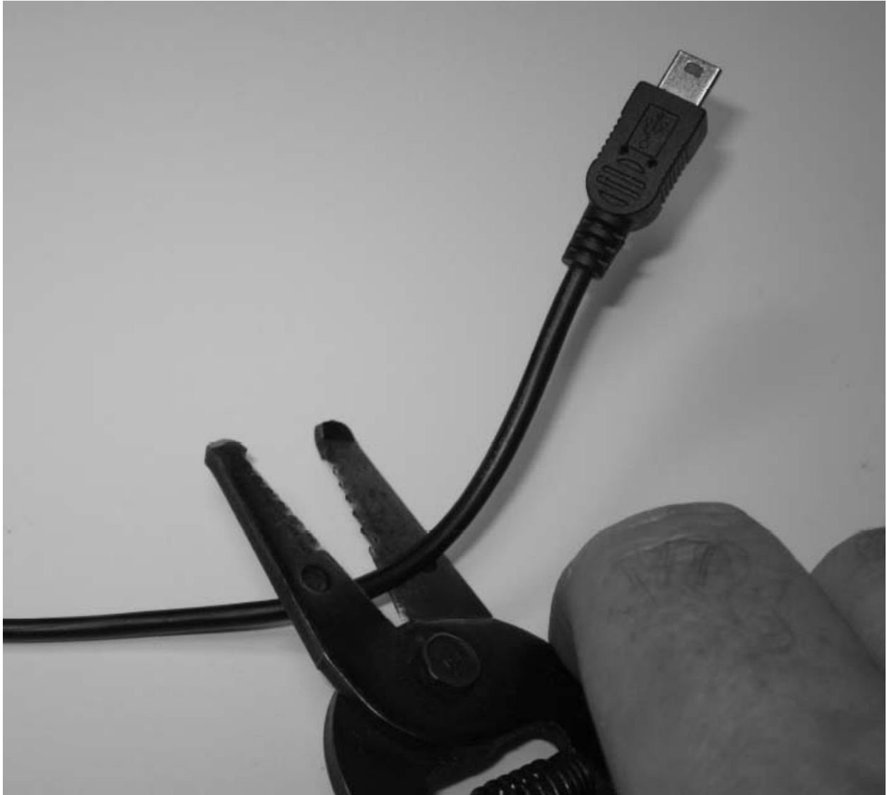
Figure A-5. Cut off the device end of the USB cable. If you cut off the wrong end, you're not going to be able to plug it back into the charger, at least not without a considerable amount of effort. To ensure you cut the correct end, plug the host end of the cable into the USB charger before snipping, and then cut off the other end.
