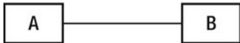
Figure 3-1. A very simple electrical schematic diagram, showing how to get from point A to point B with a single wire. Drawing wires in schematics is easy!
