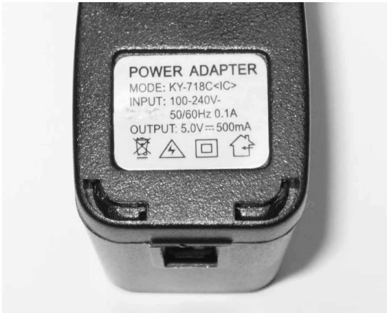
Figure A-3. The label of the USB charger tells us that it accepts anything from 110VAC to 240VAC at either 50Hz or 60Hz. This wide range of input power allows the same internal electronic design to be used worldwide. Only the prongs that plug into the wall vary from location to location. The label also tells us that the USB charger will output +5V at up to 500mA. That's 2.5W!
