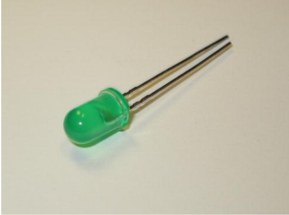
Figure 4-4. Typical LEDs in the 3mm, 5mm, 8mm, and 10mm sizes almost always have two polarity indicators. The first is that the longer lead is the positive lead, or anode (top). The second is that the flat side on the base indicates the negative lead, or cathode (bottom).
