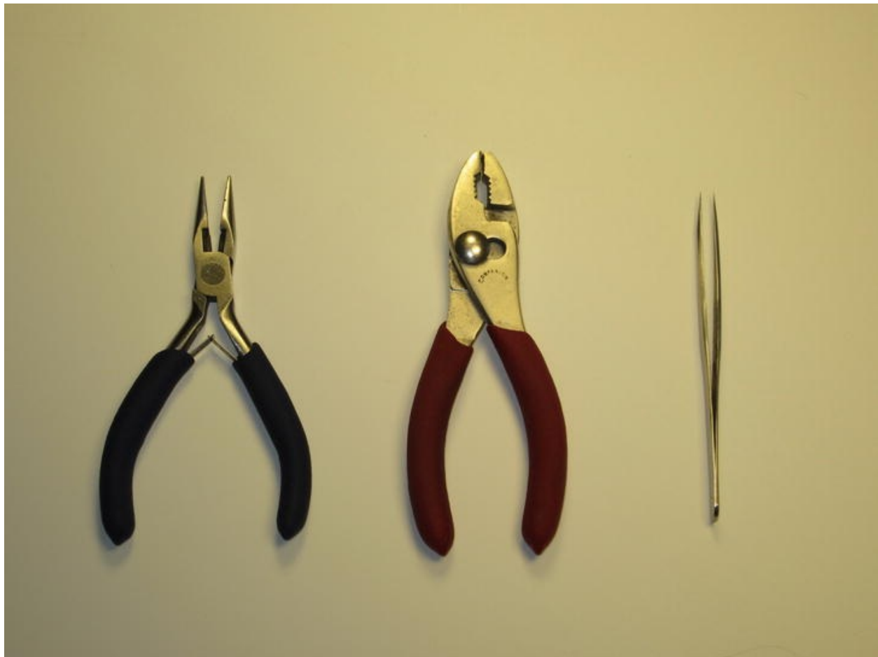
Figure 2-4. Pliers and tweezers aid in working with small parts. On the left is a pair of needle-nosed pliers with cushioned grips and leaf springs. In the center is a pair of slip-joint pliers that can be adjusted to accommodate two different ranges of gripping action. On the right is a pair of needle-sharp tweezers, which can be used to pick up and place even the tiniest of electronic components—if your hand is steady enough!
