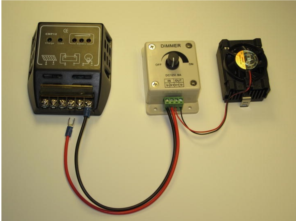
Figure 2-6. A terminal block uses a screw for tightening the connection with a bare wire.
